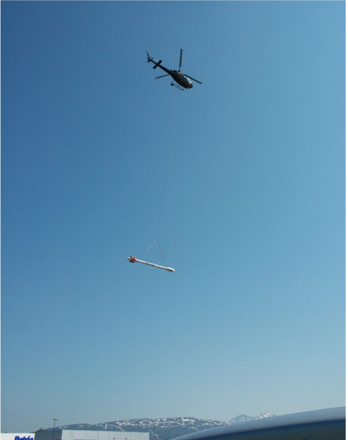
NGU measures the geophysical characteristics of the bedrock from helicopters that fly low over the terrain. Photo: NGU
