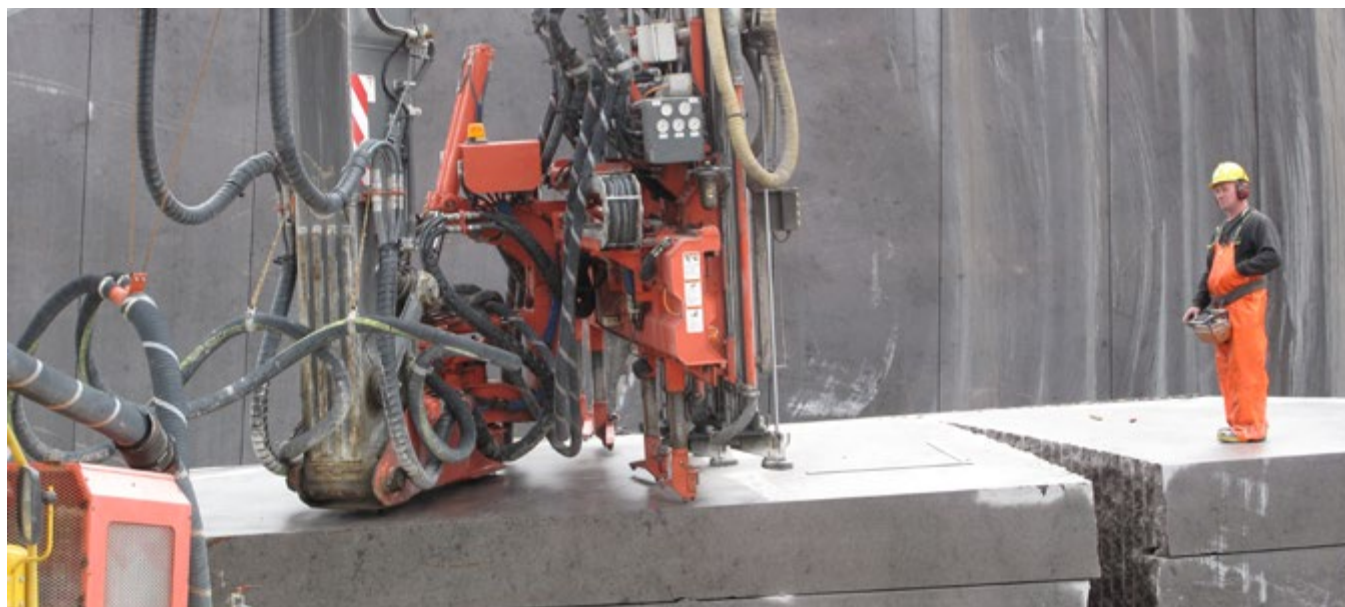
Sawing block stones, anorthosite from Sirevåg in Rogaland. Photo: Rolv Dahl/NGU
