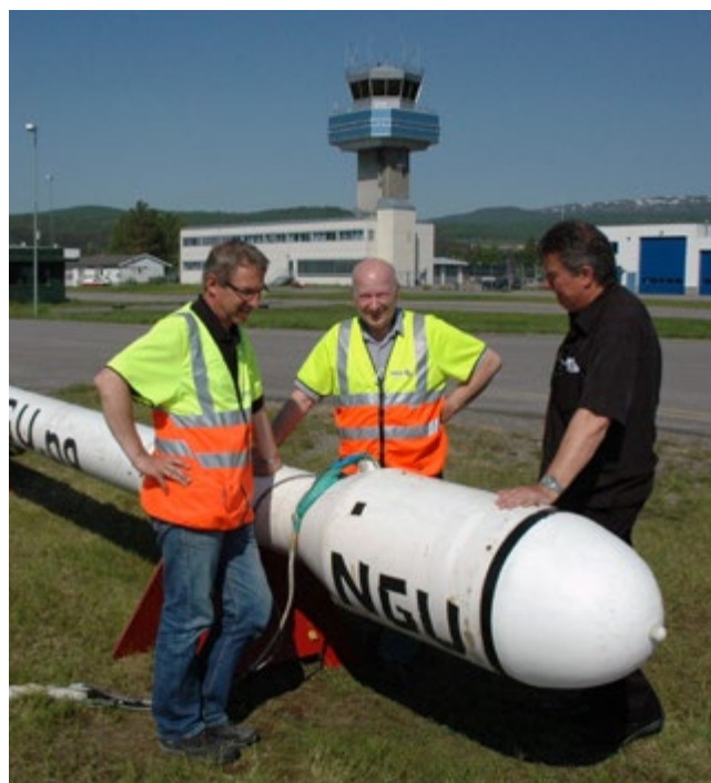
Instruments for measuring the magnetic and electro-magnetic characteristics of the bedrock are placed in a container that hangs 30 metres below the helicopter. Photo: NGU
