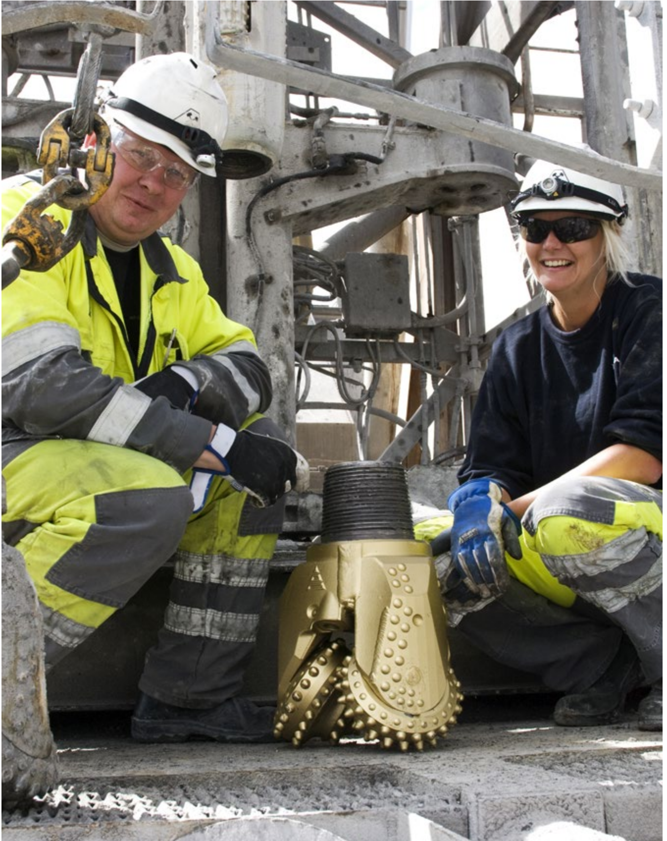
Changing a drill bit at Titania's open cast mine at Tellnes in Rogaland. Photo: Titania AS /Linda Løvås
