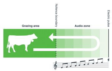
**Figure 2:** Desired response to the Nofence technology: Animal approaches virtual boundary and returns into virtual pasture upon receiving the audio cue without triggering the electric pulse.
