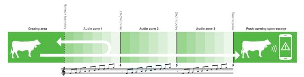
**Figure 3:** Undesired response; animal exiting the virtual boundary, triggering the escape sequence: As the animal continues out of the virtual boundary, a maximum of 3 audio warnings, each followed by an electric pulse are emitted and the escape notification is triggered.
