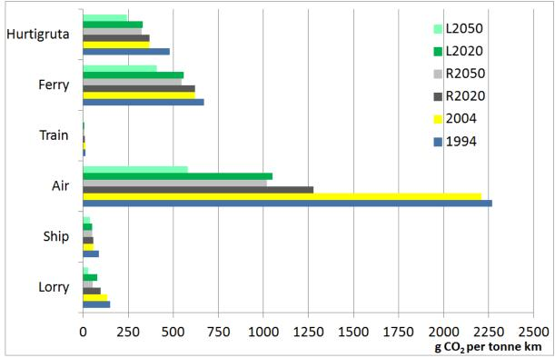
Diagram 10:  $CO_2$  emission rates for freight on Norwegian territory in 1994, 2004 and under the reference and low emissions scenarios 2020 and 2050. Source: Thune-Larsen et al. (2009).
