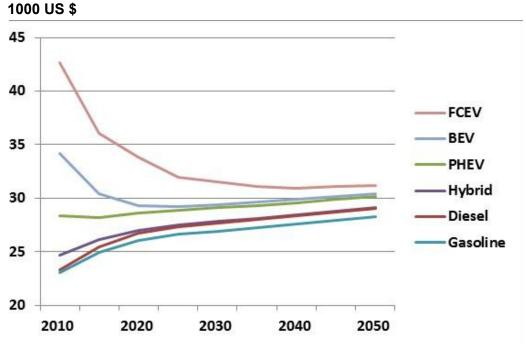
Diagram 8: Cost-based price of a representative light-duty vehicle by technology type. Source: Fulton and Bremson (2013), based on IEA vehicle cost projections.
