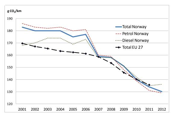
Diagram 1: Average  $CO_2$  emission from new cars registered in Norway, by fuel type, and in EU 27. Electric vehicles are included in total. Source: Fridstrøm (2012), based on input from the Norwegian Ministry of Transport and Communications, <u>OFV</u> and <u>www.eu.europa.eu</u>.
