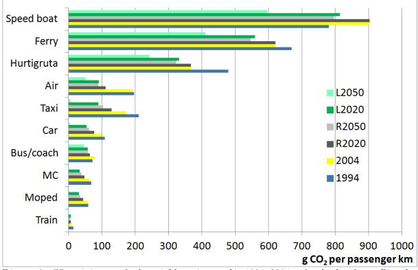
Diagram 9:  $CO_2$  emission rates for domestic Norwegian travel in 1994, 2004 and under the reference (R) and low emission (L) scenarios 2020 and 2050. Source: Thune-Larsen et al. (2009).
