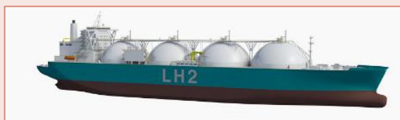
Figur 2-15: Moss Maritimes skipsdesign for flytende hydrogen.
