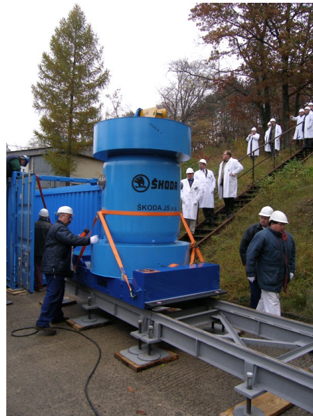
Fig.2.5 –SKODA VPVR/M cask on a rail rail-guided transfer vehicle
