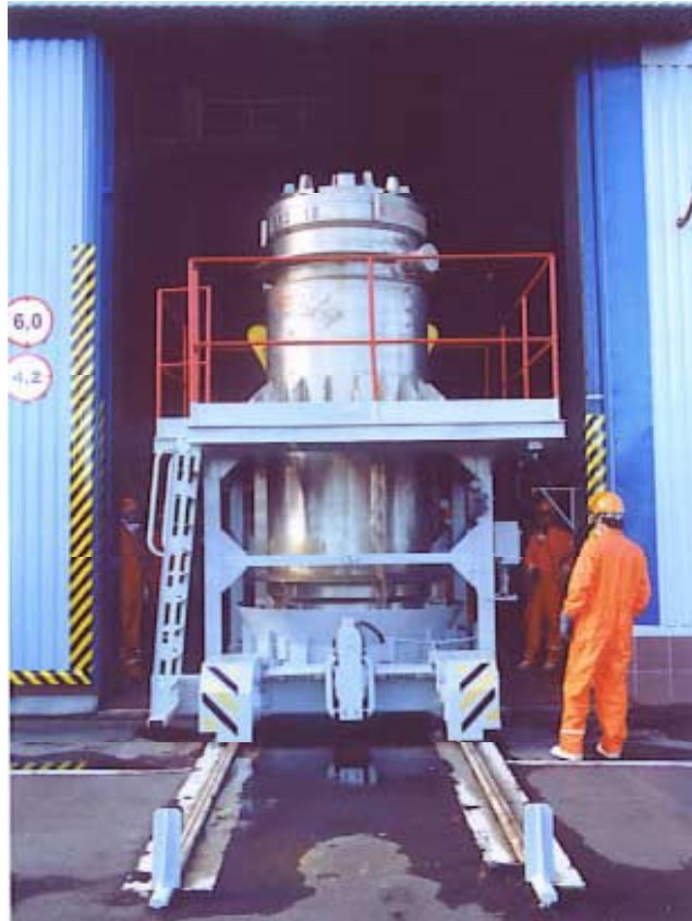
Fig.2.6 – Transfer of a TUK-18 cask on the rail-guided transfer vehicle
