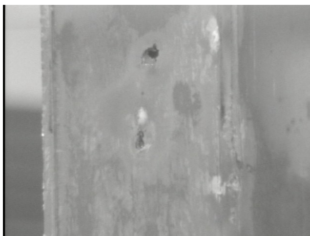
Figure 4-4. Pits through Al cladding
