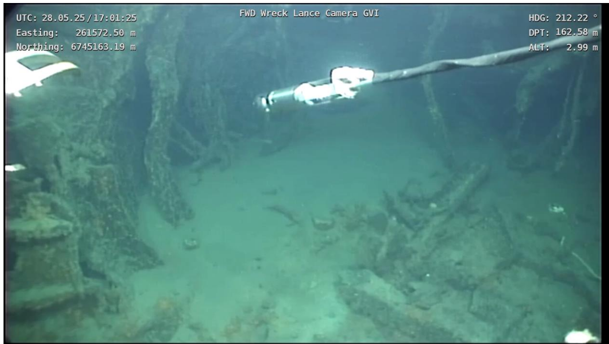
Figure 2-5 A 360° camera mounted on a lance
