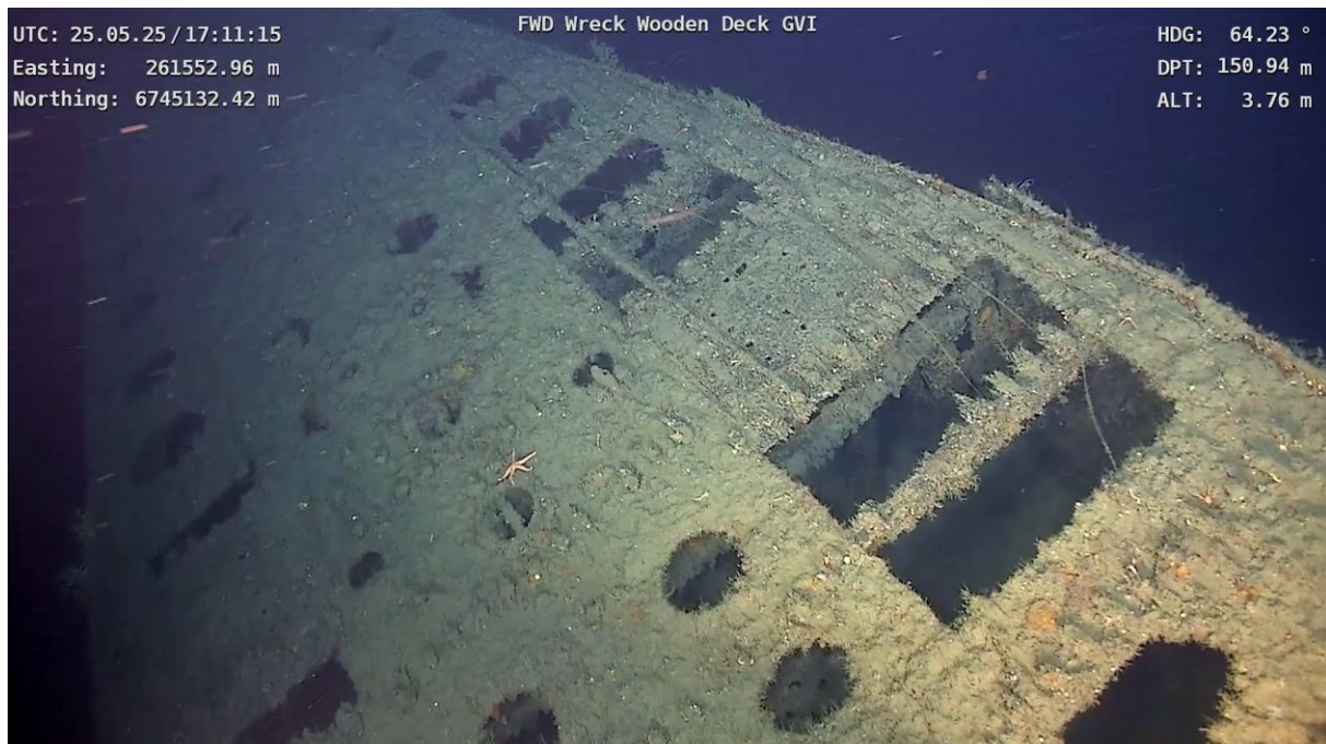
Figure 4-71 Video image example of the bow section deck with some missing panels
