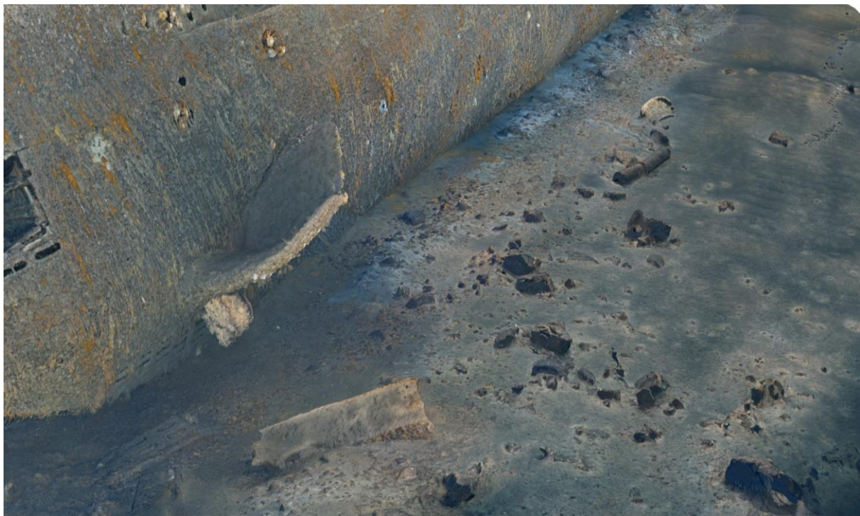
Figure 5-3 Photogrammetry data example, along the eastern side of the bow section, showing coarse sediments. The lack of submersion of debris and boulders support a coarser seabed than initially believed
