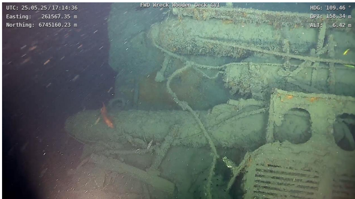
Figure 4-73 Video image example showing what is believed to be gas containers at the bow fracture point
