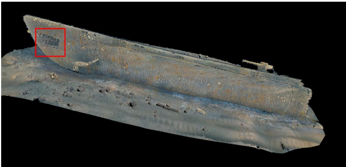
Figure 4-30 Port side view of the bow section showing missing panels at the front
