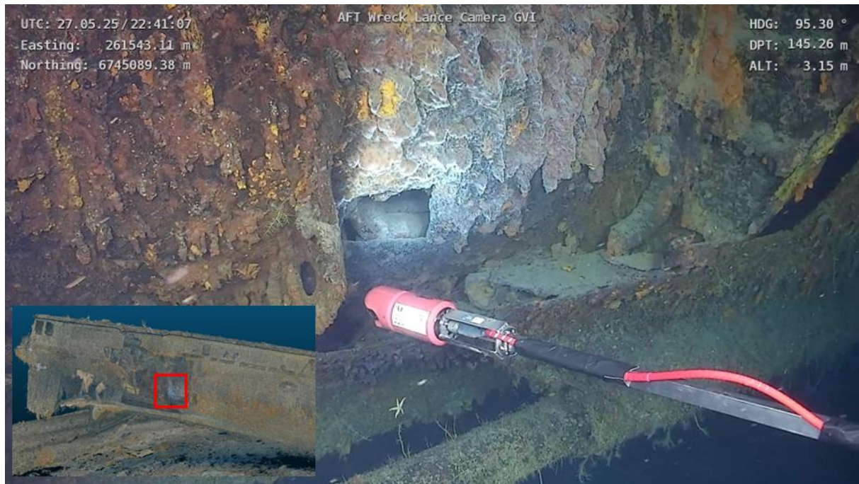
Figure 3-22 ROV camera example showing the lance camera before entering the hull
