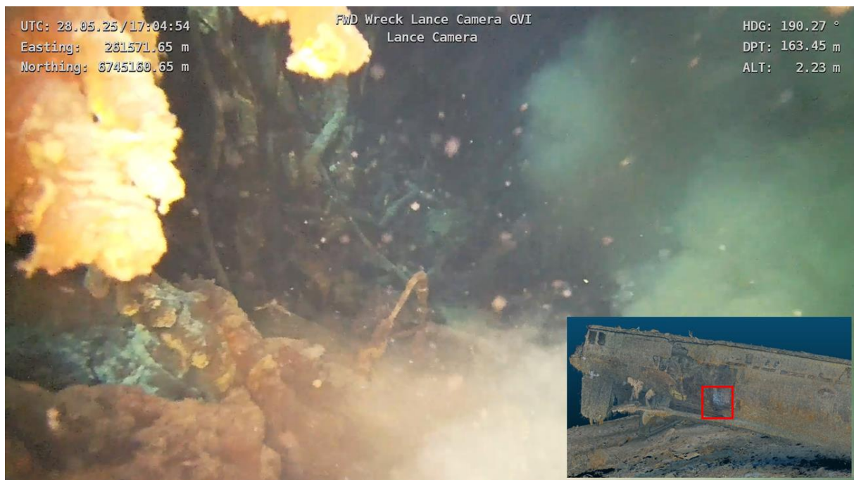
Figure 3-19 Lance camera example showing suspended material obstructing the view
