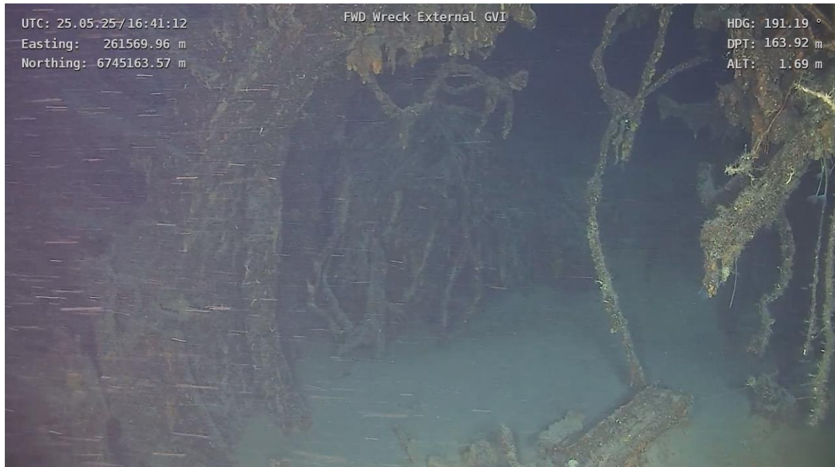
Figure 4-59 Video image from the bow fracture point showing debris blocking the entrance
