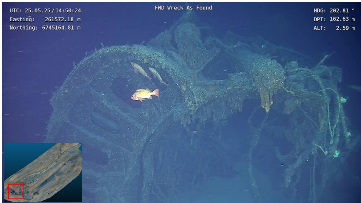
Figure 4-33 Bow section fracture point showing damages. Significant sedimentation is seen within the opening
