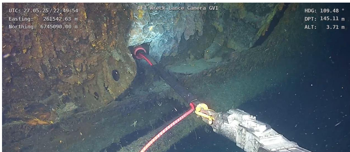
Figure 4-68 Video image example showing the lance camera inserted into the cut-out location
