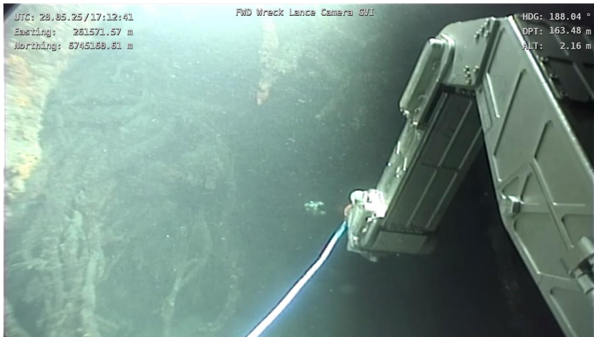
Figure 4-60 Video image showing the lance camera extended into the bow fracture point
