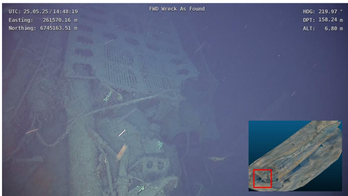
Figure 3-17 HD video example from the bow fracture point
