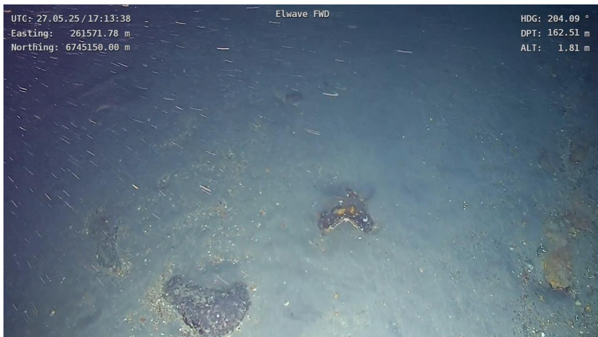
Figure 4-23 Video image of the magnetic anomaly. It is most likely some debris
