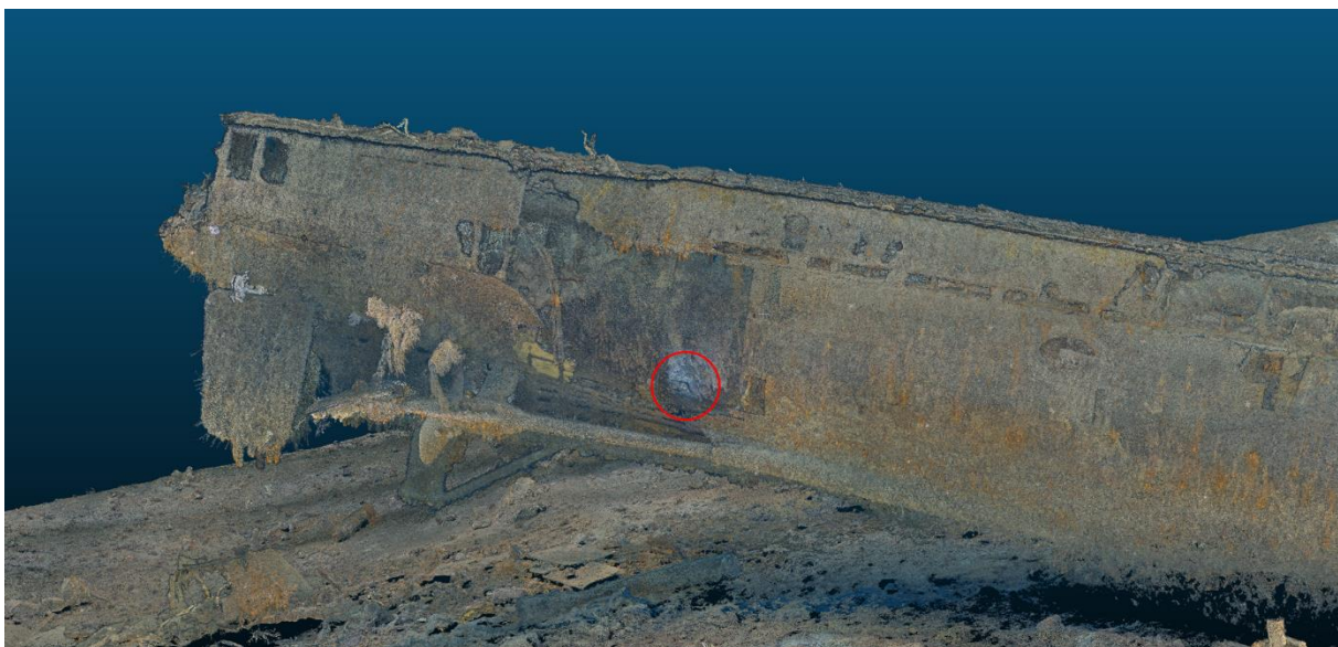
Figure 4-64 Photogrammetry model showing the location of the cut-out where the lance was inserted
