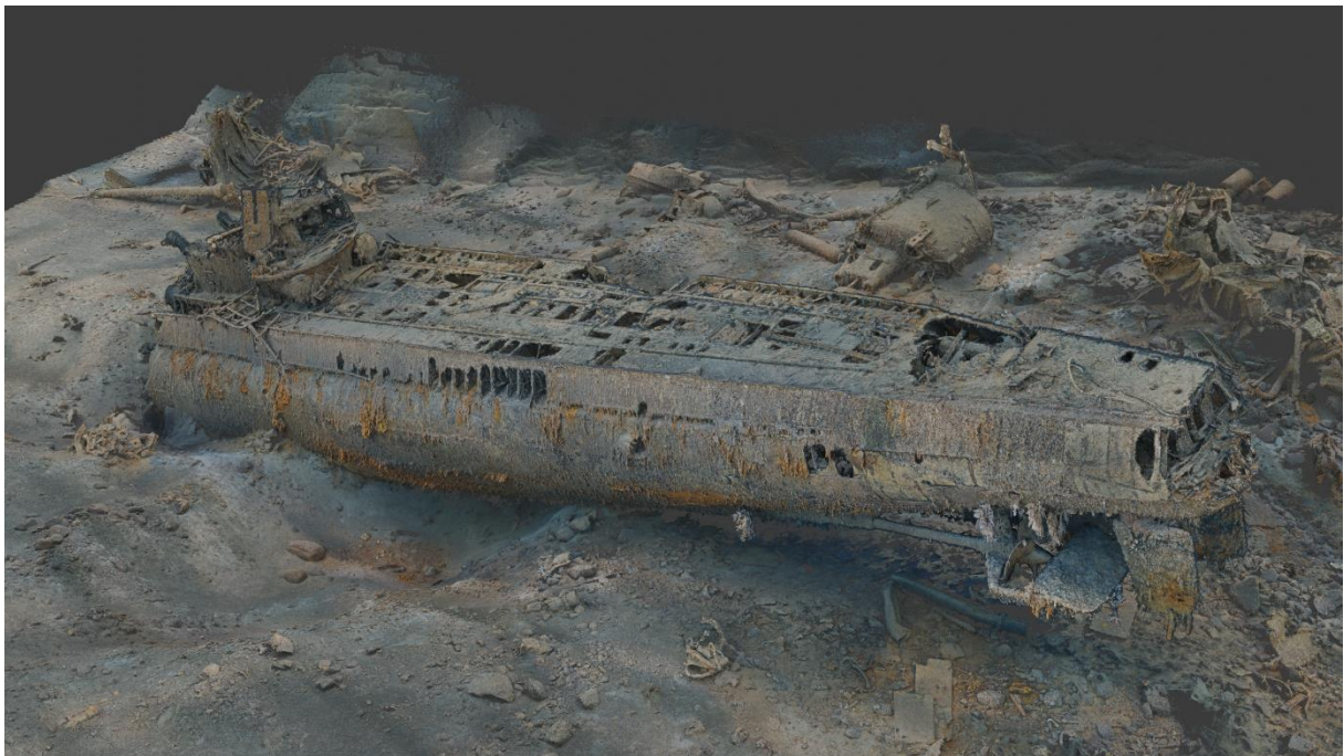
Figure 3-15 Point cloud of the stern section of U-864
