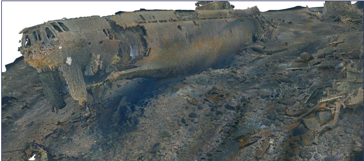
Figure 5-4 Photogrammetry data example, of the stern section, showing coarse sediments. The lack of submersion of debris and boulders support a coarser seabed than initially believed
