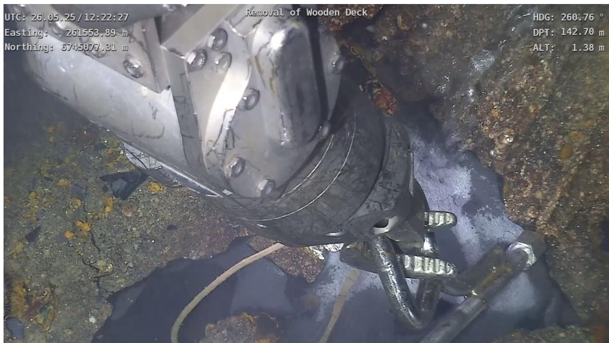
Figure 4-86 Bubbles emanating from the cylinder just above the manipulator
