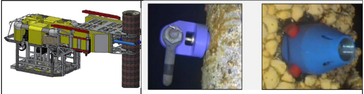
Figure 6-3: The Core drilling (left side) can be executed by WROV holding it, or more advanced by the placement of a jig with core driller inside, to be adjusted to its relevant position on the submarine. The lower right pictures shows a conductor lifting pin c/w 35Te shackle and locking dogs activated. Can be applied for the M1: roll method.
