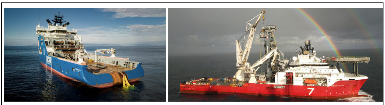
Figure 8-15: Left picture shows the AHTS Horizon Arctic, and the Right picture shows HCV Seven Arctic. The latter vessel is equipped with a 900T HC crane.
