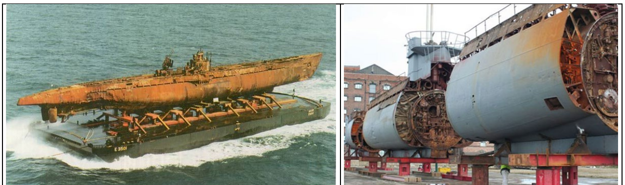
Figure 8-2: Submarine U-534 of type IXC/40 had a displacement of 1,144 tonnes. It was initially recovered in one piece but was later cut into five larger sections of maximum 240
