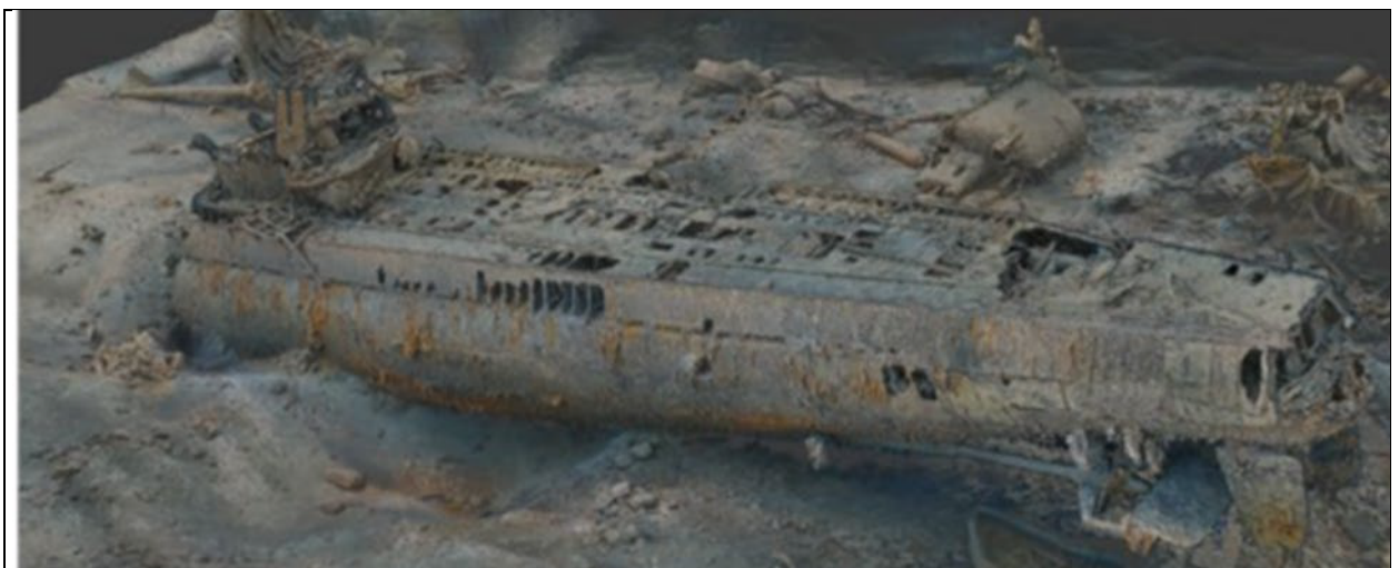
Figure 8-10: The situation for the stern section is different for the stern section as for the bow section. For the stern section, the nearest bulkhead is crushed, leaving the interior more exposed to inflow of sediments.
