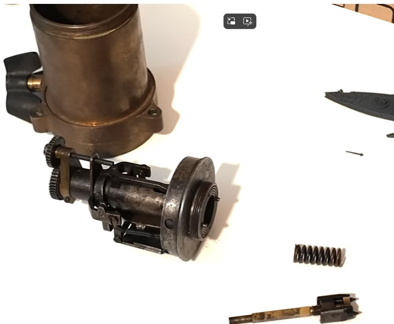
Figure 3-5 Overview of all components inside the torpedo detonator
