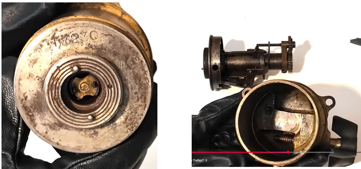
Figure 3-3 Right: Top lock of firing device including firing pin. Left: inside housing with grease firing device in the background
