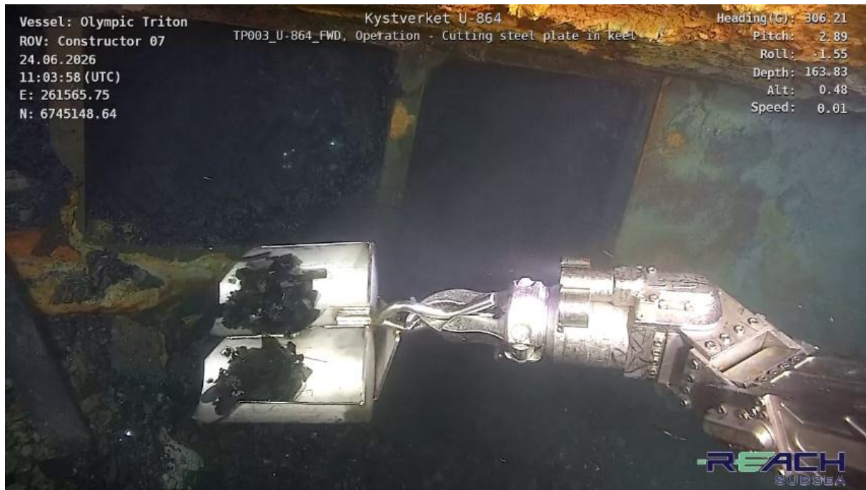
Figure 3-40 Inspection of keel compartment at frame #60
