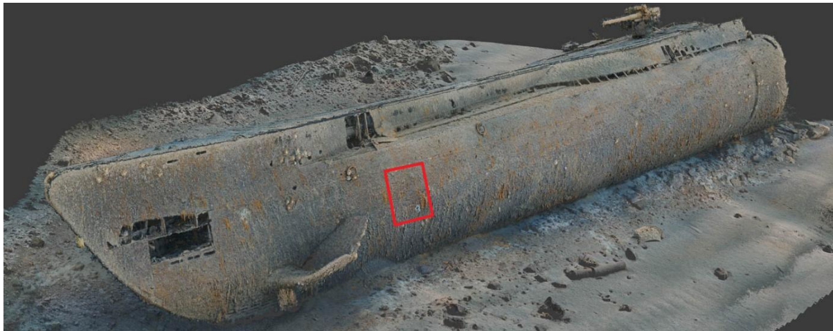
Figure 3-35 Approximate location of cutting for FMD works
