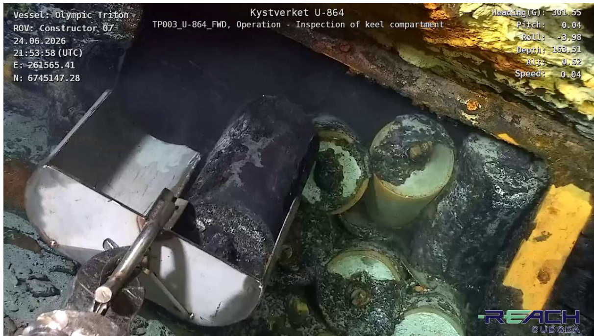
Figure 3-22 Recovery of mercury canister from keel compartment frames #65-#66 (#110-#112)
