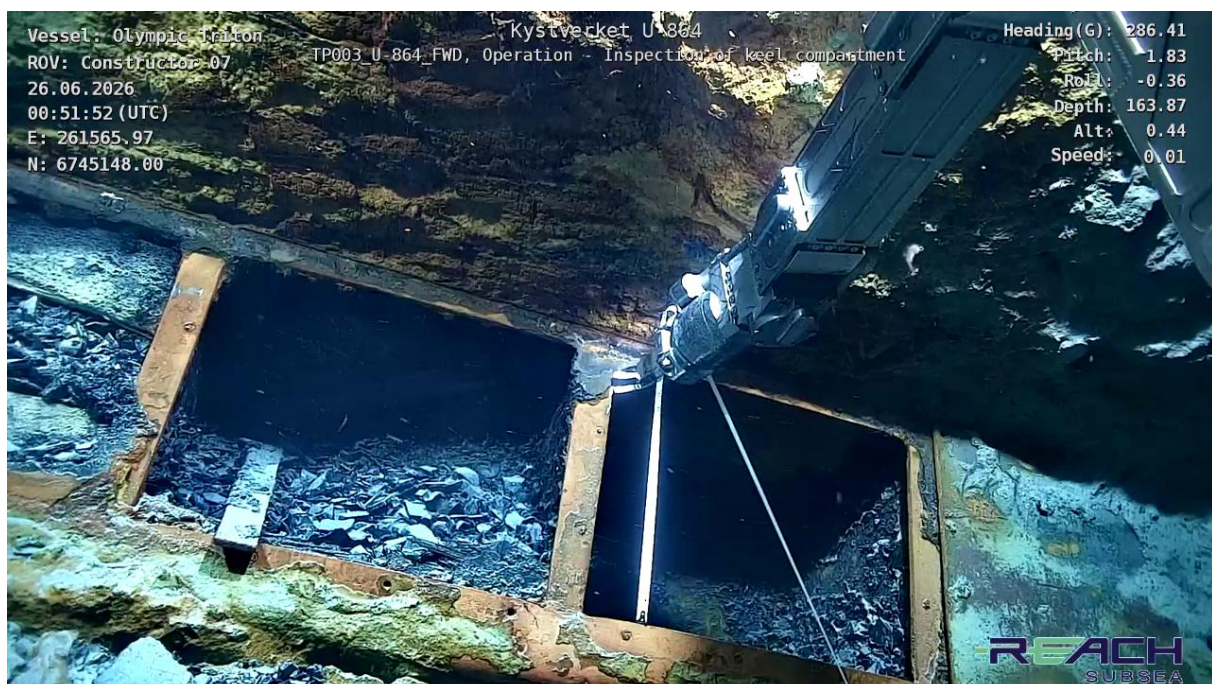
Figure 3-43 Measurements of the canister compartment aperture - He 50cm - Width 62cm - Depth 50cm
