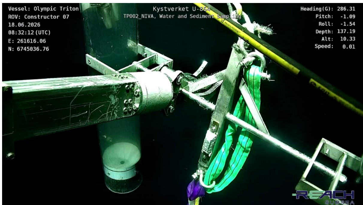
Figure 3-5 Cleaning sediment traps (Tp-002)
