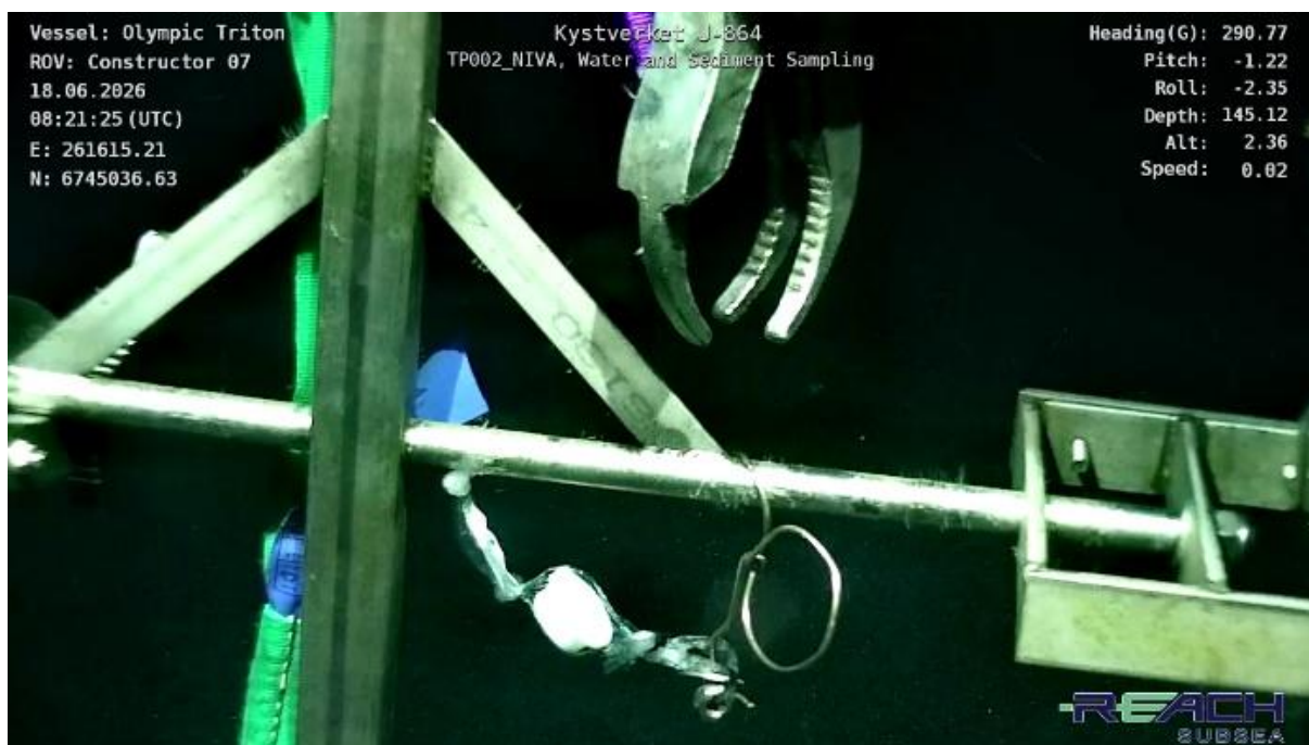
Figure 3-7 DGT bag installed on sediment trap
