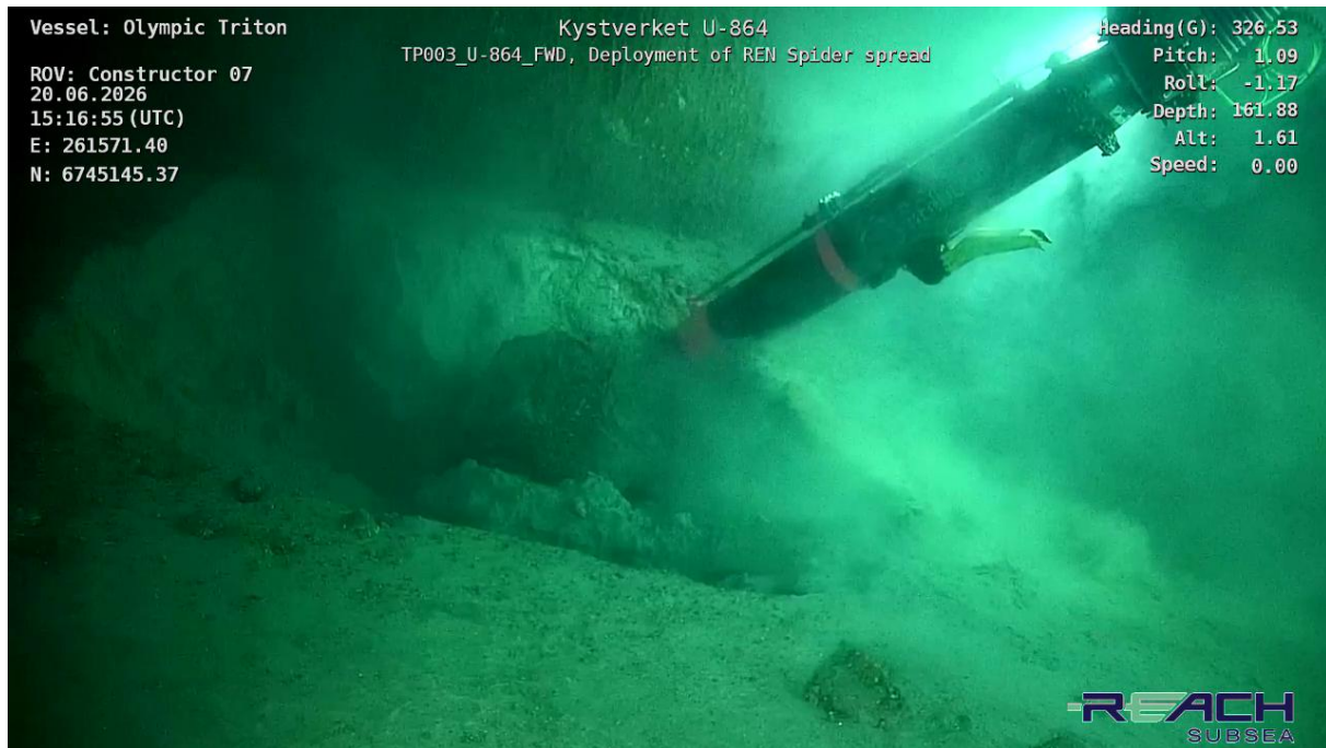
Figure 3-15 RenOcean Spider dredging operations
