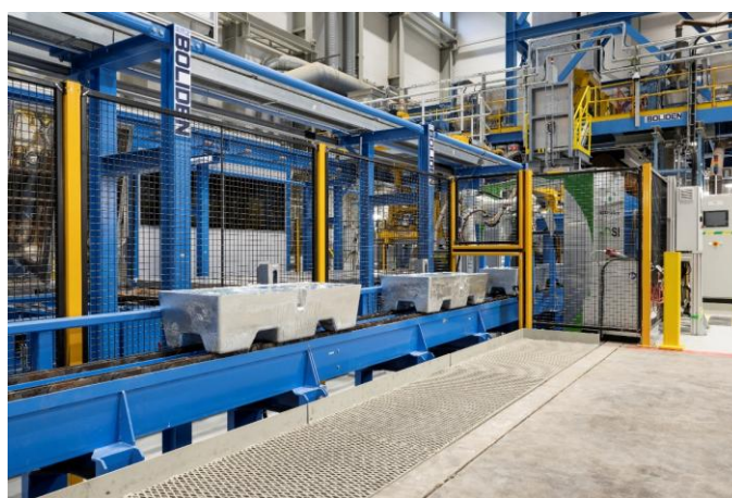
Figure 26 - Transport of cast products at a fully automated zinc foundry at Boliden Odda. (Photo: Thor Brødreskrift)
