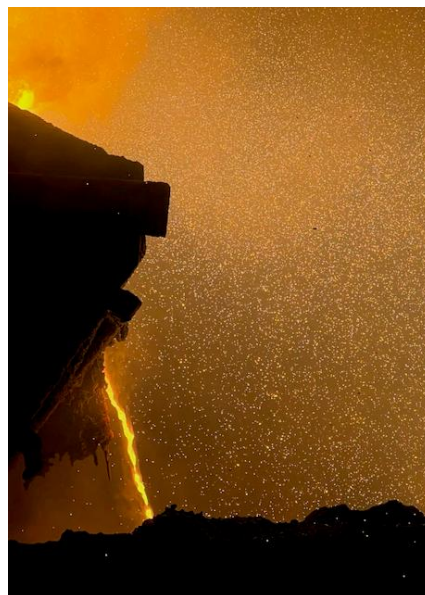
Figure 44 - Pouring of ferrosilicon metal at the Finnfjord smelter. (Photo: Finnfjord)
