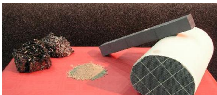
Figure 49 - Silicon carbide primary material, submicron powder and example of a product for use in filtration. (Photo: Washington Mills)
