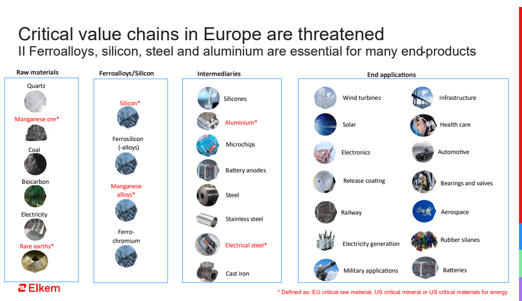
Figure 29 - Slide from Elkem showing raw materials for silicon (Si) and ferrosilicon (FeSi) production. Si and FeSi form part of alloys in various semi-finished products such as aluminium profiles or electrical steel. (Source: Elkem)
