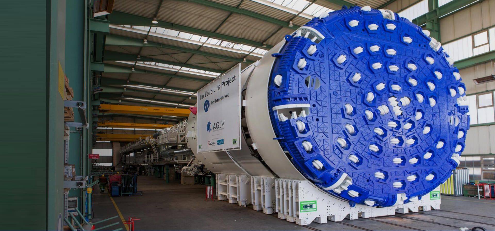
The first of four TBMs designed for abrasive and strong Norwegian rock (Herrenknecht, Germany)
