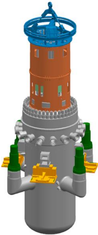
Figure 2.15: The Integrated RPV for the ACP100 SMR (CNNC, 2023)
