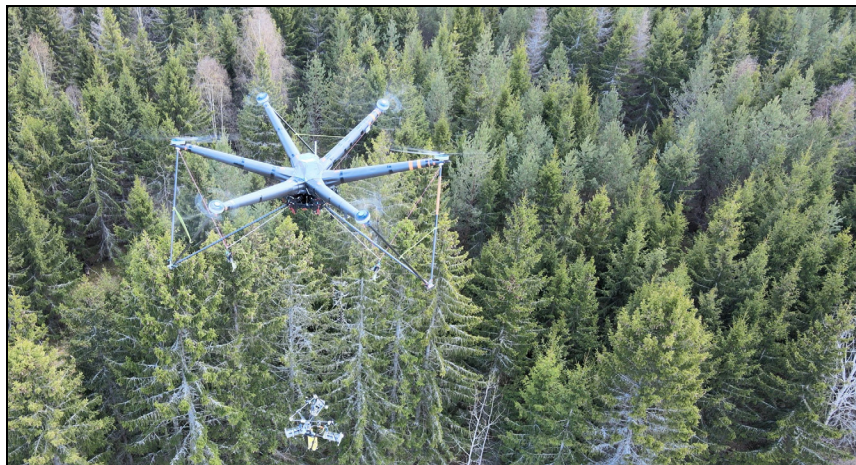
Figure 7.1 Forest thinning operation using a drone with attached cutting device
