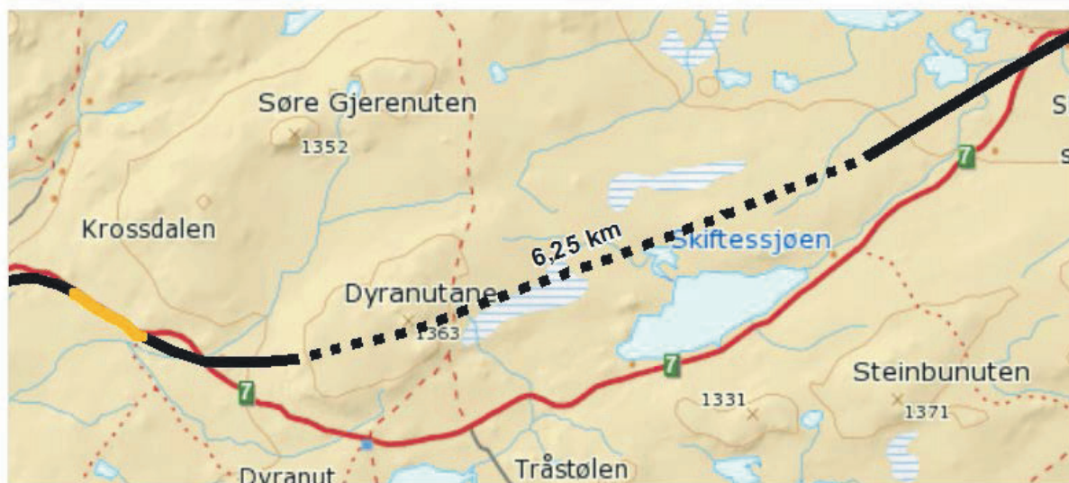
Figur 23: Konsept K2 Dyranut-tunnel
