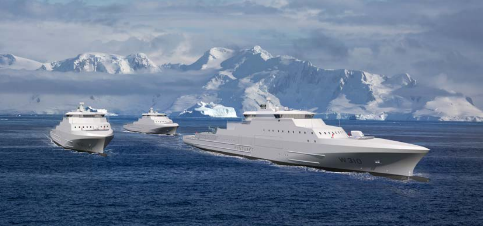
The Vard Langsten shipyard in Møre og Romsdal is to build three new Coast Guard vessels (length 136 metres and beam 19 metres), which will carry up to 100 people. Illustration: Vard.
