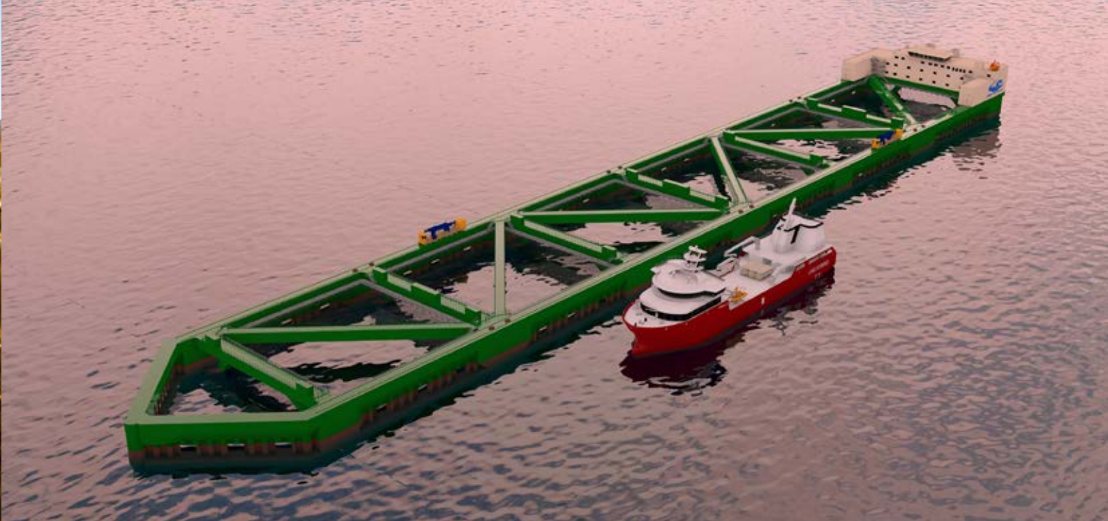
Nordlaks has been granted funding from Innovation Norway to develop Havfarm, a new type of fish farm. The company has also been granted development licences from the Ministry of Trade, Industry and Fisheries. This innovative fish farm can be sited in exposed waters, and is designed to withstand wave heights of up to 10 metres. Photo: Nordlaks/NSK Ship Design.
