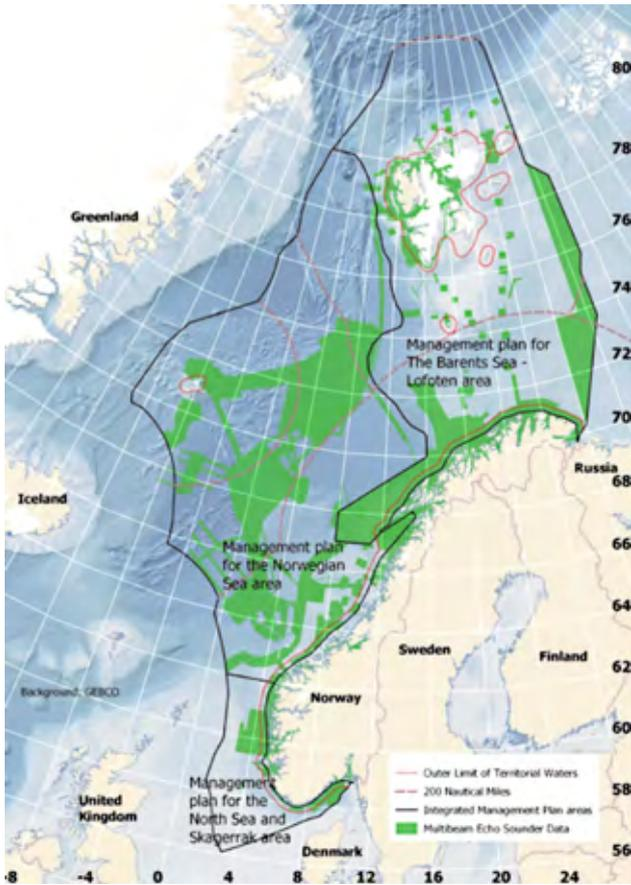
Surveys by the Norwegian seabed mapping programme "Mareano" (in the Exclusive Economic Zone incl some international waters Banana hole). Detailed terrain models of the seabed exist for the green areas. Terrain models are based on data from surveys with multi beam echo sounders from surface vessels.
