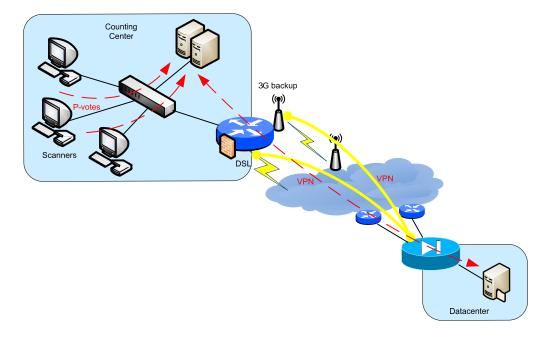
Only the server of the counting center will have access to the datacenter. The firewalls will allow only desired ports after the decryption of the VPN.
