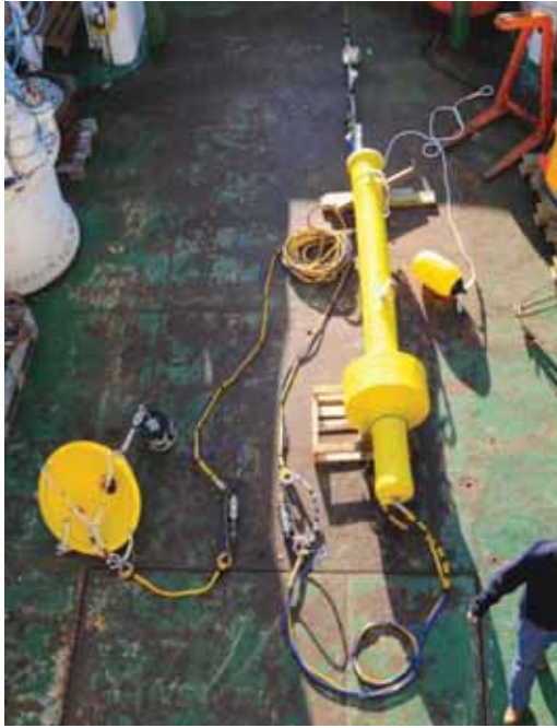
Figur 2.6. Hydrofonbøye med to hydrofoner (Hydrophone buoy with two hydrophones.)
