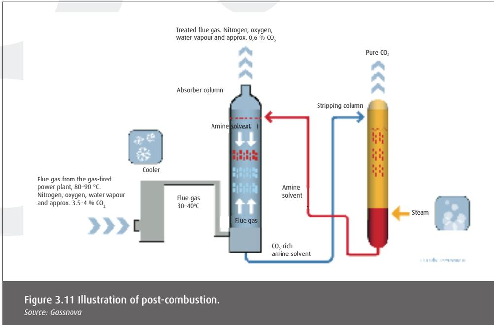
Figure 3.11 Illustration of post-combustion.
