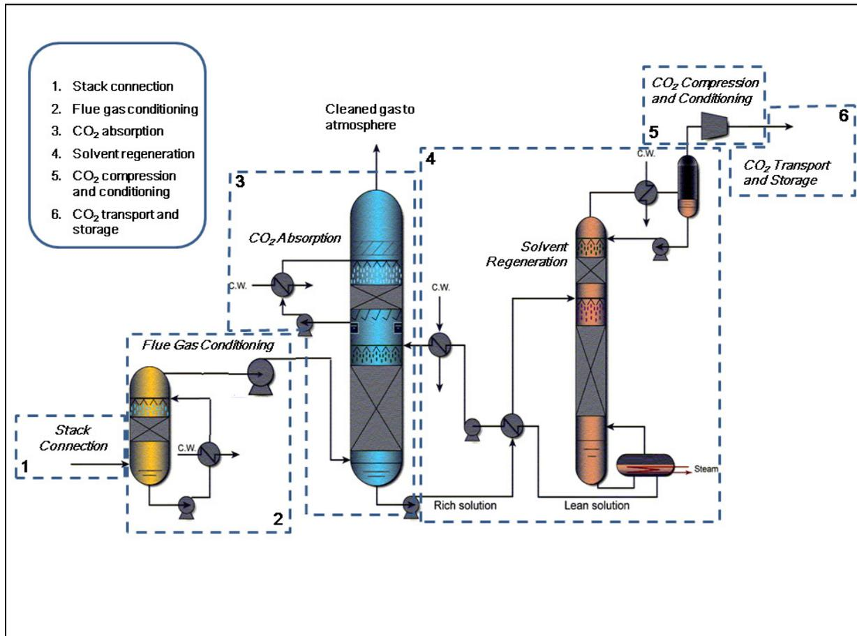
Figure 3-3 Typical amine based carbon capture and compression plant (Source: SINTEF)
