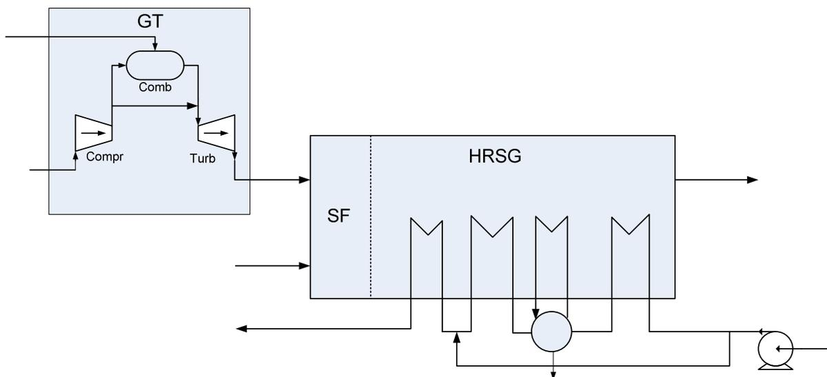
Figure 10-1 Gas turbine and heat recovery unit model
