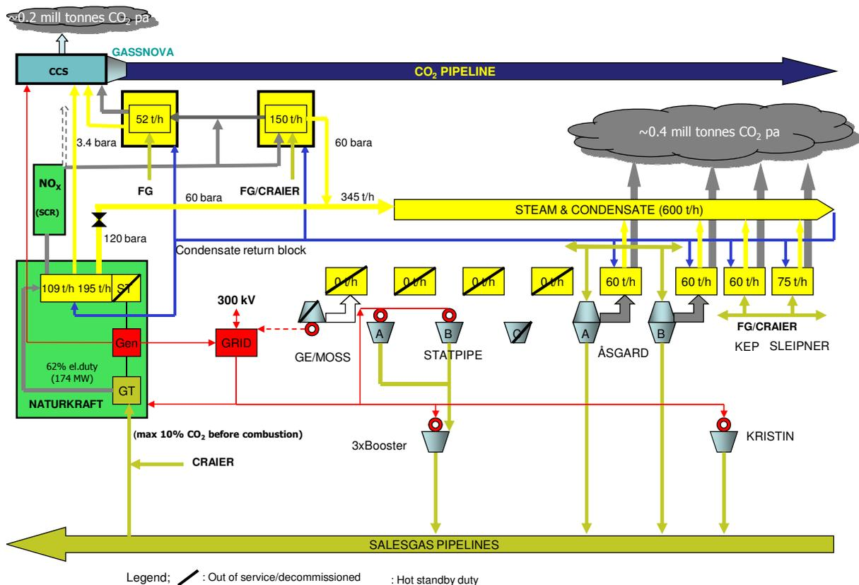
Figure 6-7 Schematic overview of scenario 4
