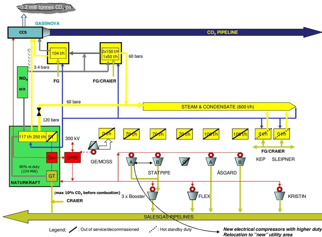
Figure 6-8 Schematic overview of scenario 5d
