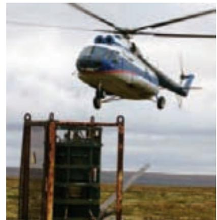
At inaccessible locations, the RTGs must be shipped out using helicopters. Photo: County Governor of Finnmark.
