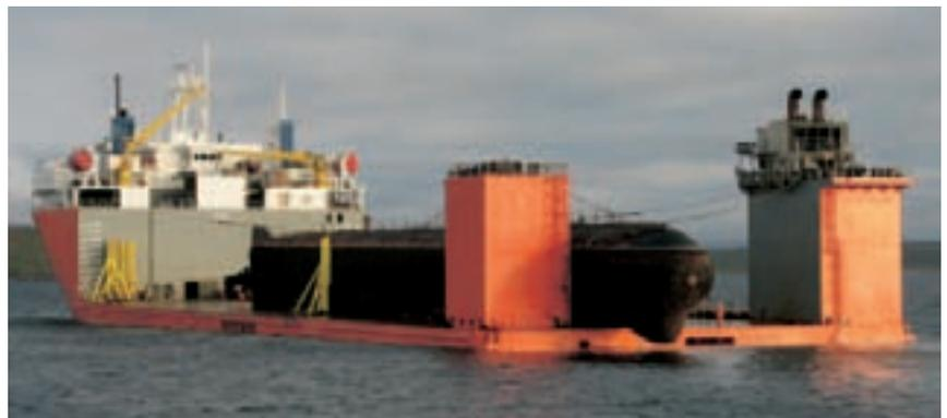
Submarine 291 on the deck of the Transshelf, ready to be secured. Photo: The Norwegian Defence Research Establishment (FFI).
