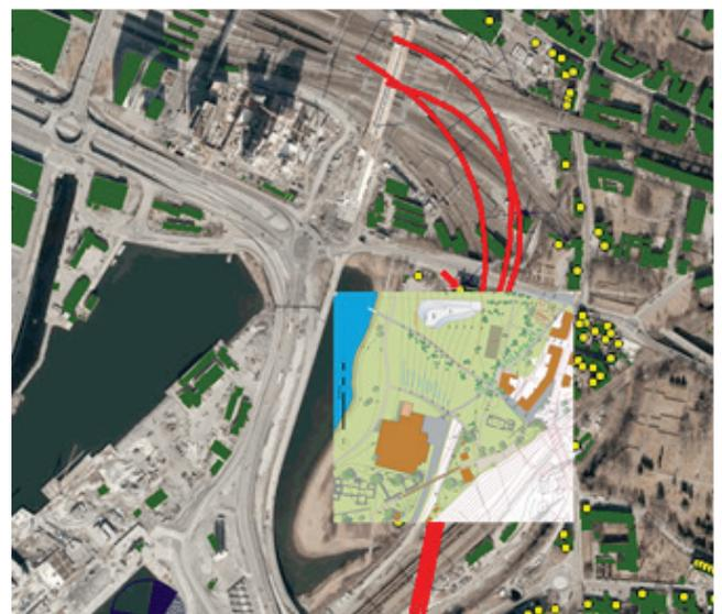
**Figure 2-5 Proposed location of new Museum Building and possible conflict with planned rail tunnel with alternative tracks in red on picture to the right (illustration by LPO architects and Jernbaneverket)**
