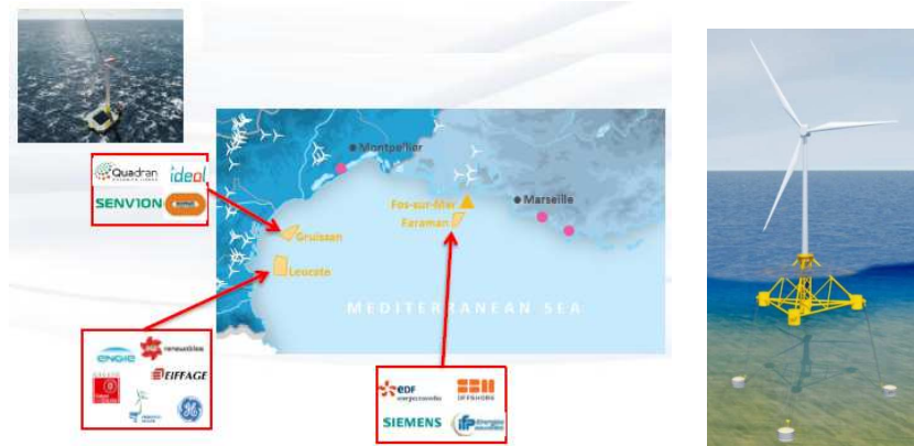
Fig. 14. (left) Mediterranean pilot farms locations and partners, (right): TLP structure (by SBM) chosen for the Provence Grand Large project at Faraman site, the only of the pilot to use 8MW turbines. Source: Pole Mer Méditerranée/EdF.
